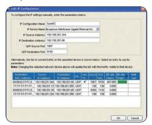
UDP sessions carrying MPEG TS traffic are indicated and may be selected for analysis and recording. Transport Stream packets are time-stamped as they are received from any Network Interface Card, allowing PCR measurements and graphing to be supported both on the MTS4SA Series instruments and on a user's own PC.
